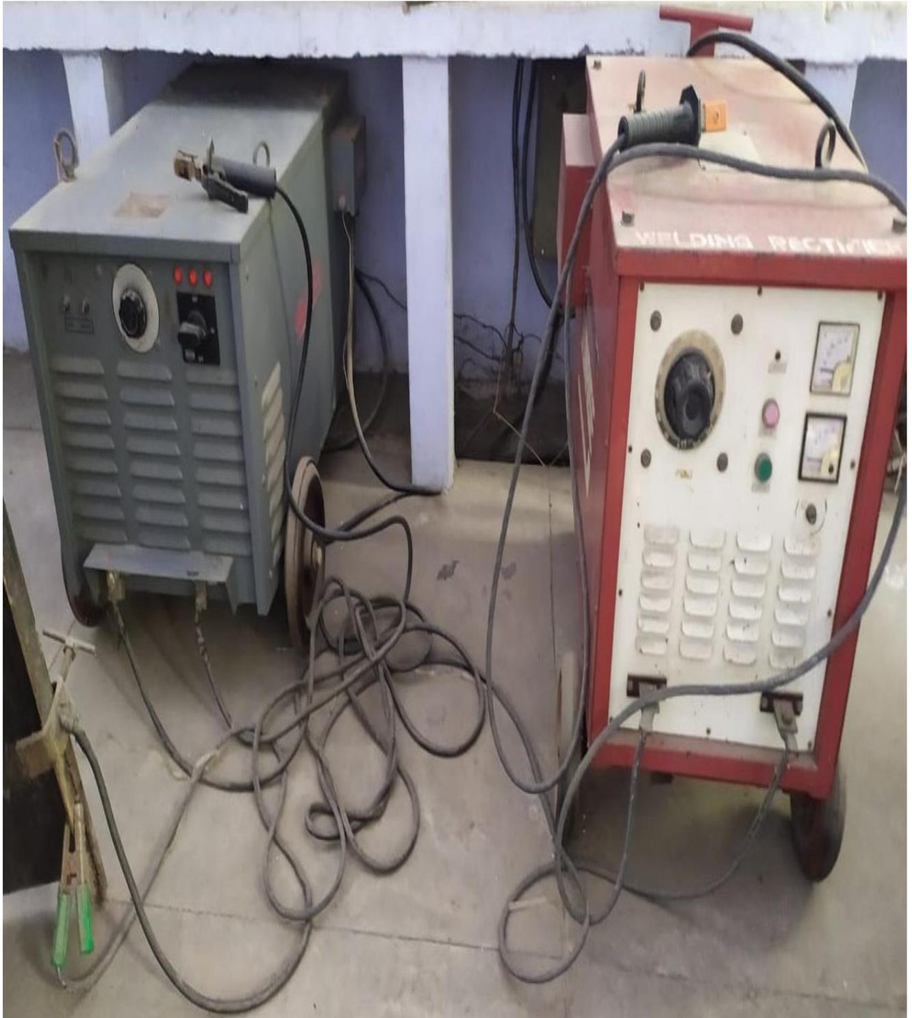
Welding Transformer and Rectifier
